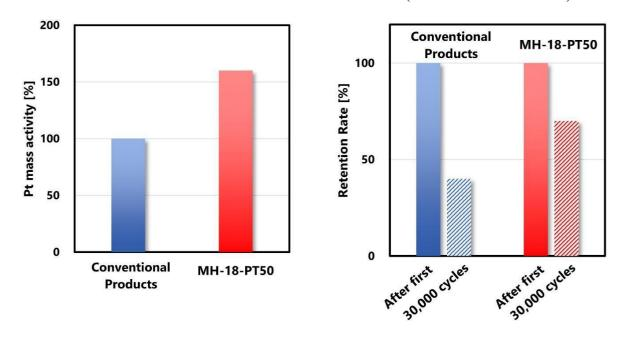
%1: Measurement results with Anode/Cathode = H2/O2, MEA Cathode
