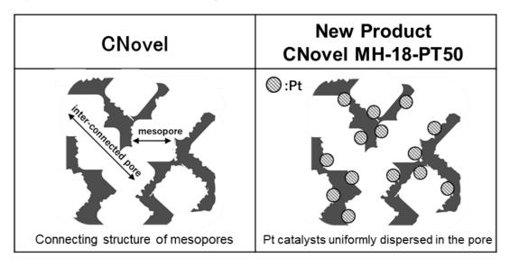
Fig.1 Illustration of CNovel<sup>TM</sup> (mesoporous carbons) and Pt-loaded CNovel<sup>TM</sup> "MH 18 PT50"
