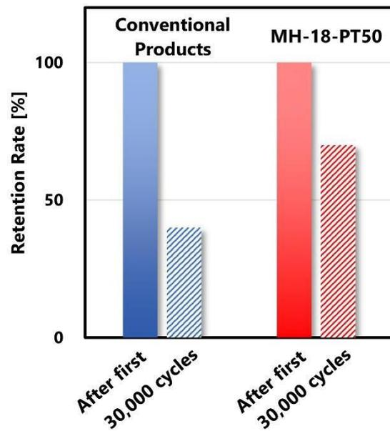
※ 1 : Measurement results with Anode/Cathode = H<sub>2</sub>/O<sub>2</sub>, MEA Cathode
